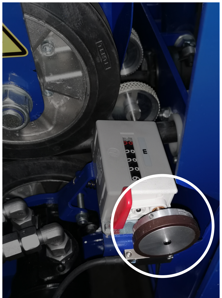
Tachometer. This sensor is connected to the meter counter and, when rotated, gives a signal to the control board about the movement of the rinsing pipe. If the sensor is damaged or loose, the pipe feed system will malfunction, and the pipe feed auto-pilot function will not work.
