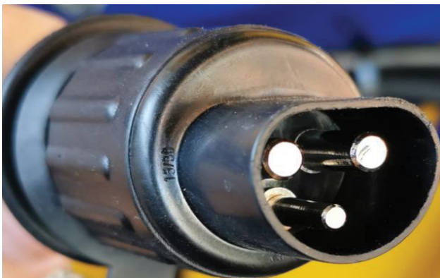
Electrical connection plug-in for control unit. This plug-in is for connection to the tractor power supply. If the control unit is not connected to power, the remote control system will not operate. The control unit needs to be supplied with 12 V.
